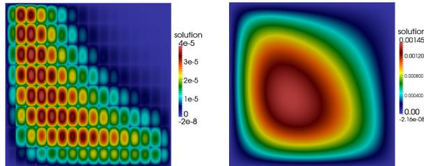
**Fig. 1** Numerical solutions obtained by Schwarz parallel additive algorithm in 2D on 128 processors(1 subdomain/processor): First schwarz iteration(Left) and solution at convergence(Right)
