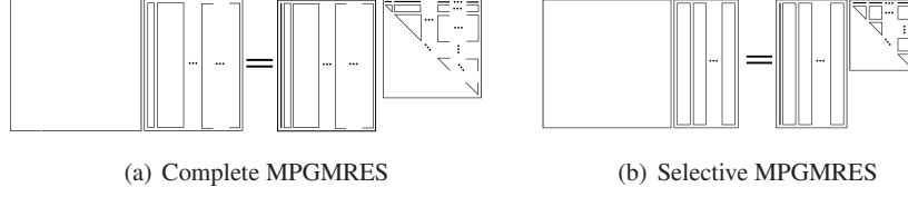
Fig. 1 Schematic of Arnoldi decompositions in complete and selective MPGMRES
